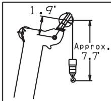
NOTE: 1. Boom and jib geometry shown are for unloaded condition and machine standing level on firm supporting surface. Boom deflection and subsequent radius and boom angle change must be accounted for when applying load to hook.
